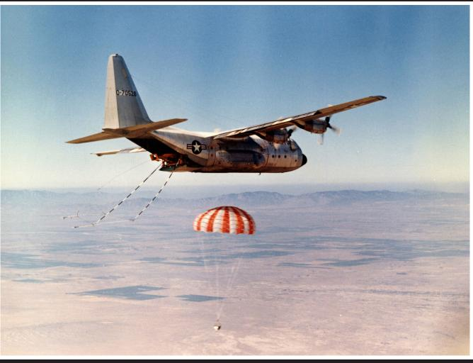
> JC-130 aircraft recovering parachute with test payload.
