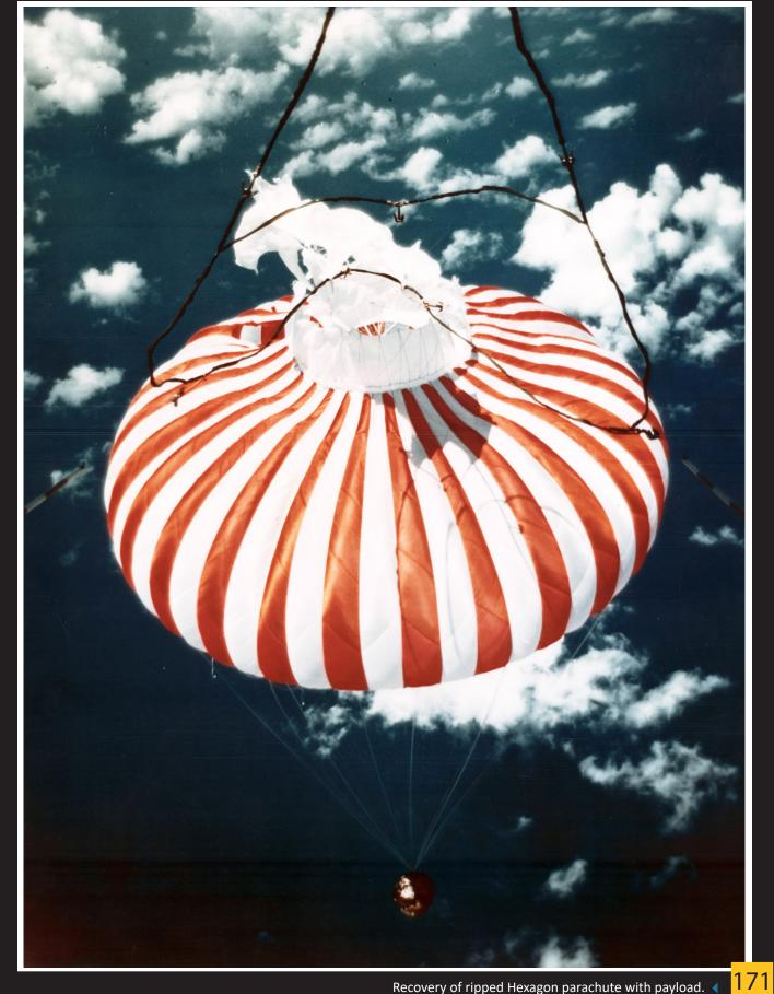
170 • Hexagon Mark VIII recovery parachute and film canister.
