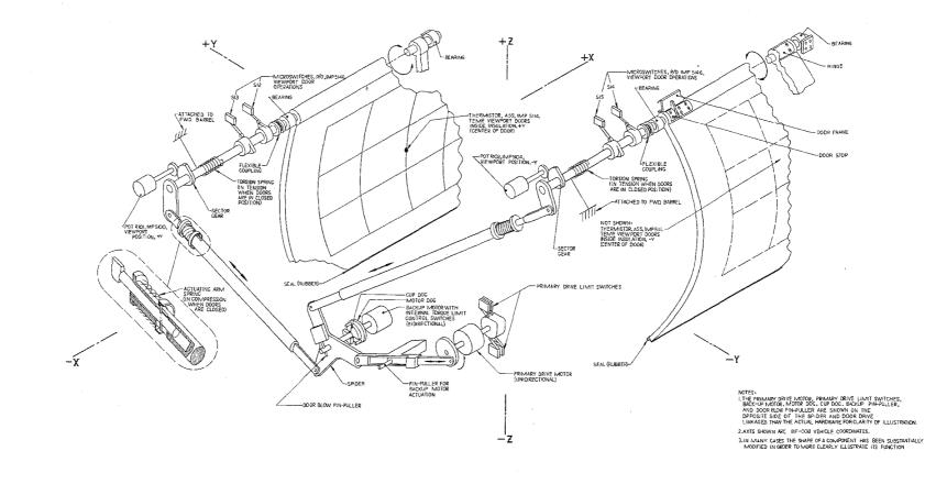
Figure 3.5-3. Viewport Door Drive Mechanism and Instrumentation
