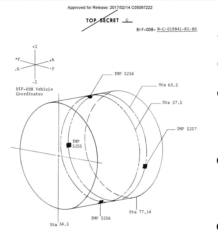
Figure 3.8-16. Supply Electronics Module Skin Temperature Instrumentation Points
