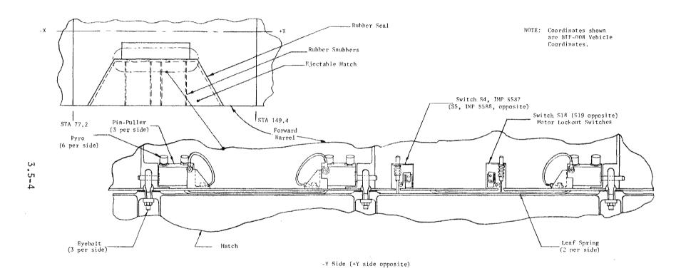
Figure 3.5-2. Hatch Ejection Mechanism
