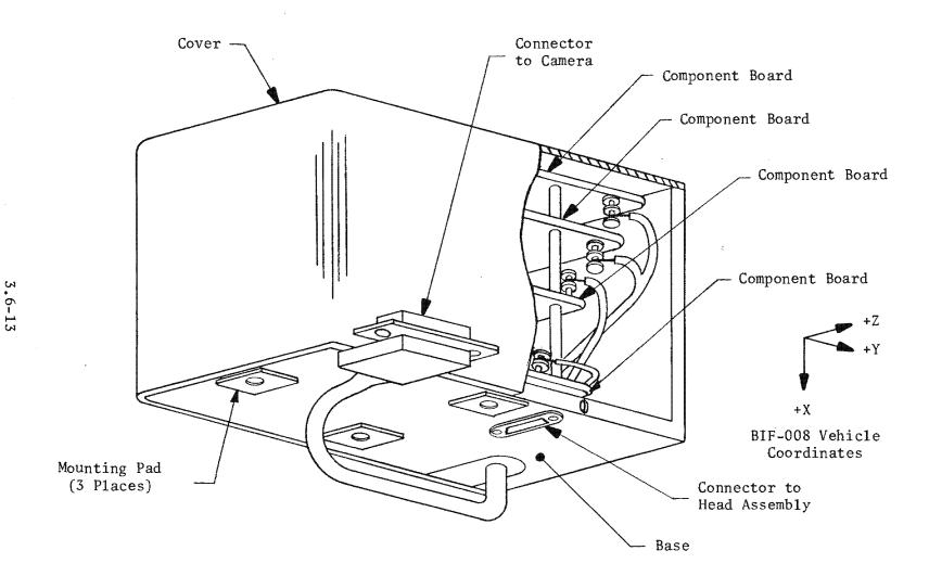
Figure 3.6-9. Instrumentation and Control Module (Unit 15A1)
