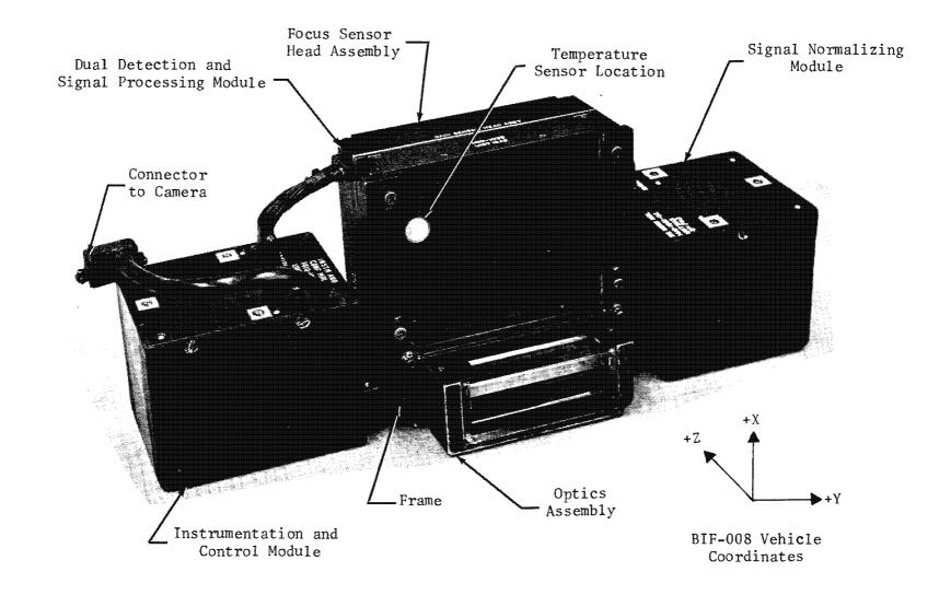
Figure 3.6-1. Focus Detection Subsystem Elements
