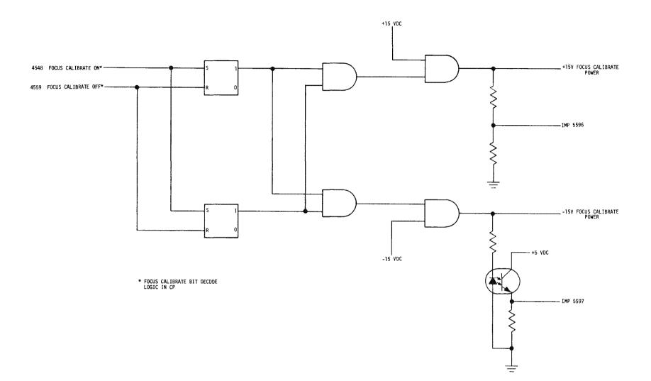
Figure 3.7-9. Focus Detection Subsystem Calibration Power
