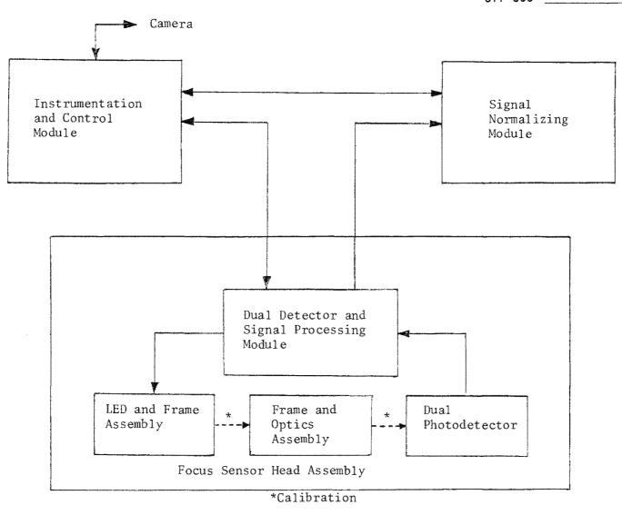
Figure 3.6-3. Focus Detection Subsystem Block Diagram
