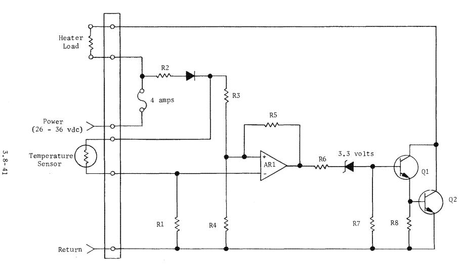
Figure 3.8-9. Ground Heater Controller Schematic
