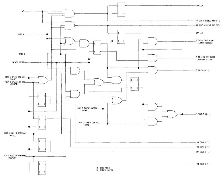
Figure 3.7-28. 5 Splice and Cut and 5 Roll-In Terminate
