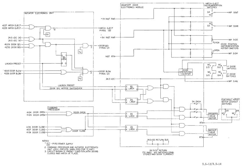
Figure 3.5-5. Viewport Door Subsystem Electronics
