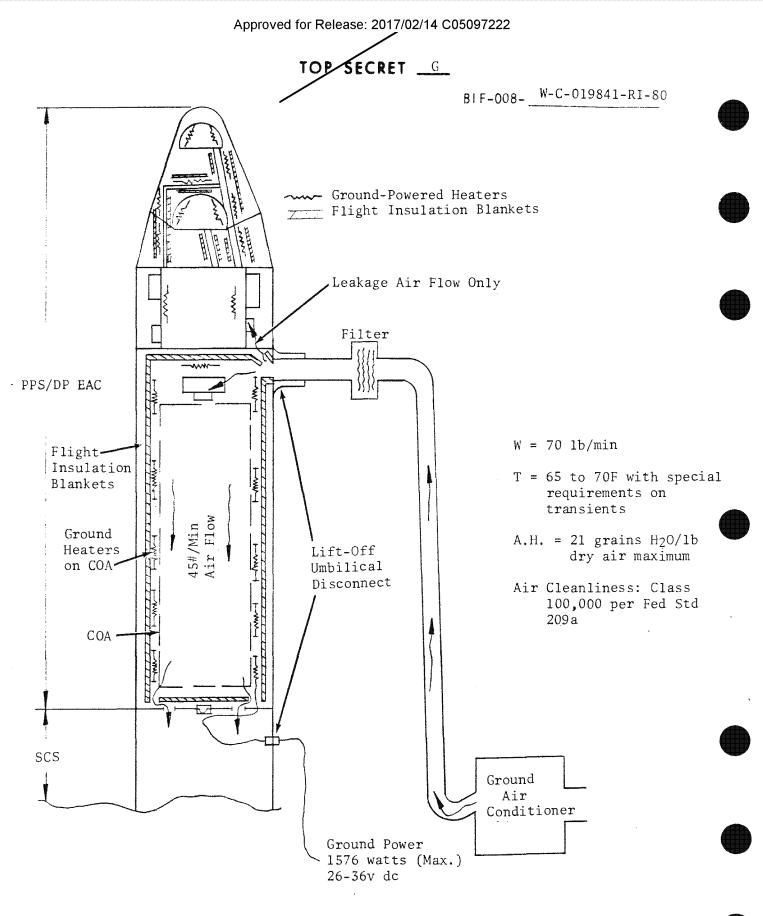
Figure 3.8-2. PPS/DP EAC On-Pad Conditioning System
