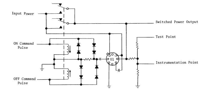
Figure 3.7-14. Standard Soft Switch Circuit
