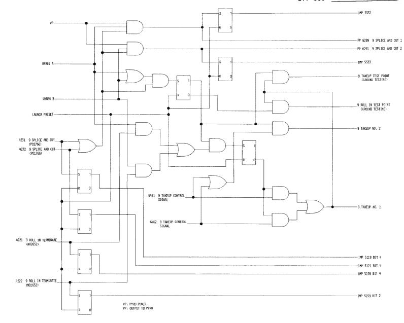
Figure 3.7-27. 9 Splice and Cut and 9 Roll-In Terminate
