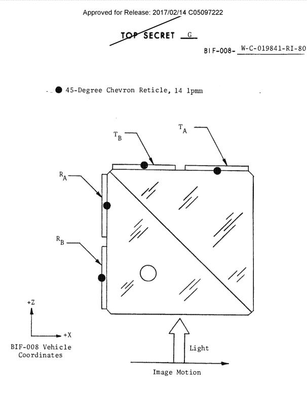
Figure 3.6-6. Beam Splitter and Reticle Assembly
