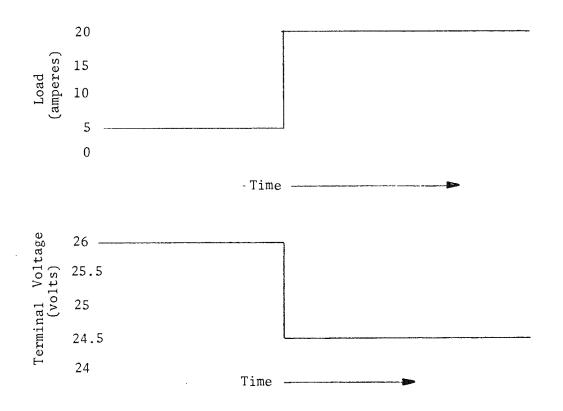
Figure 3.7-4. Voltage/Load Relationship Due to Solar Panel Effect
