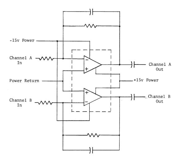
Figure 3.6-15. Typical Dual Channel Amplifier
