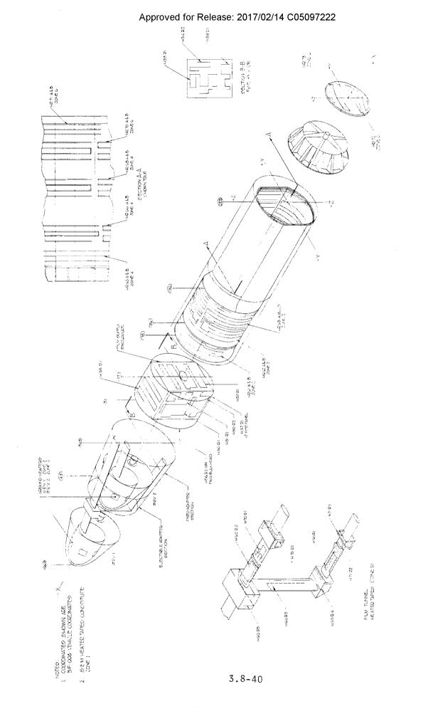
Figure 3.8-8. Ground Heater Tape Locations
