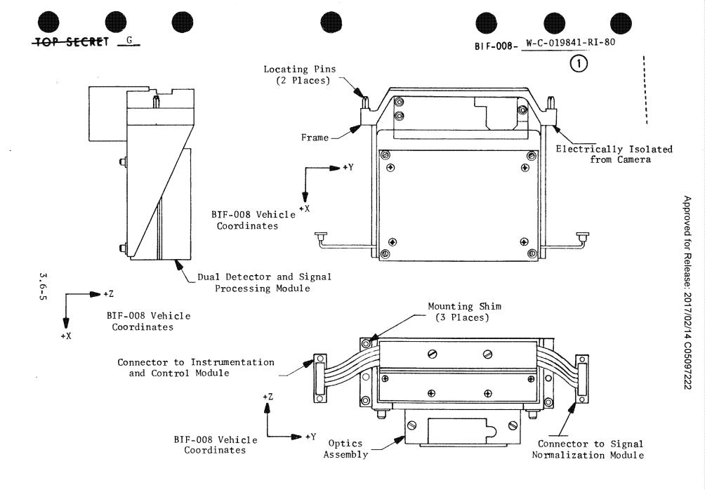
Figure 3.6-4. Focus Sensor Head Assembly "WARNING - THIS DOCUMENT SHALL NOT BE USED AS A SOURCE FOR DERIVATIVE CLASSIFICATION"
