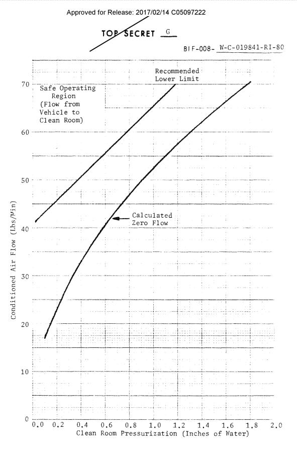
Figure 3.8-4. Recommended Operating Limits for Clean Room
