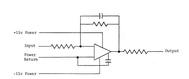
Figure 3.6-17. Typical Scaling Amplifier and Low-Pass Filter
