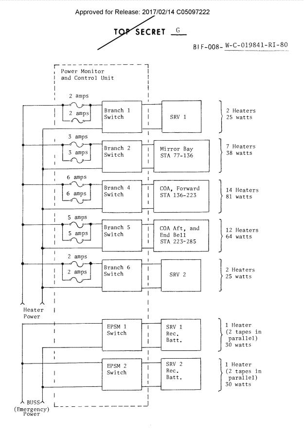
Figure 3.8-10. Flight Heater Branch Block Diagram
