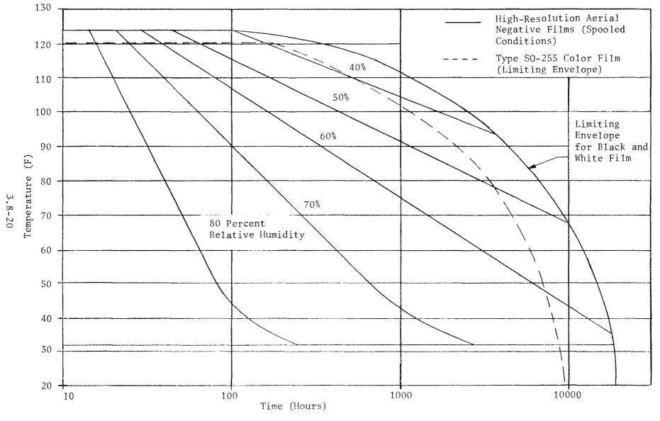
Figure 3.8-5. Film Temperature vs Time Keeping Limits
