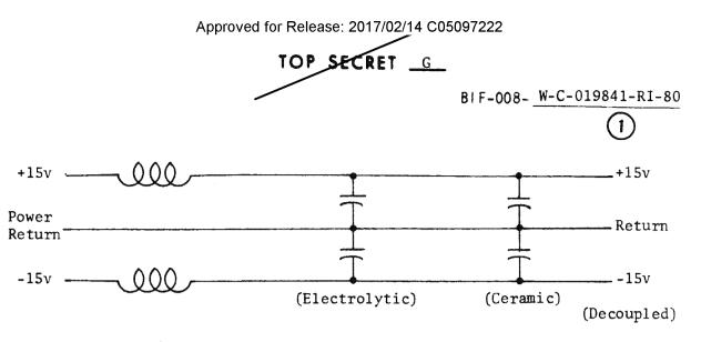
Figure 3.6-20. Power Decoupling Circuit
