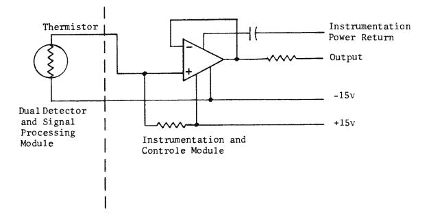
Figure 3.6-19. Temperature Sensor Bias Network
