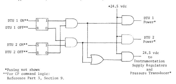
Figure 3.10-23. DTU Power Control Logic
