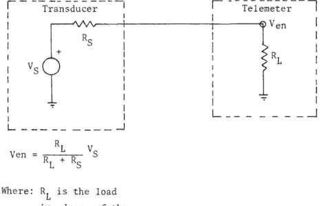
L impedance of the Telemeter and R<sub>S</sub> is the source impedance of the Transducer.
