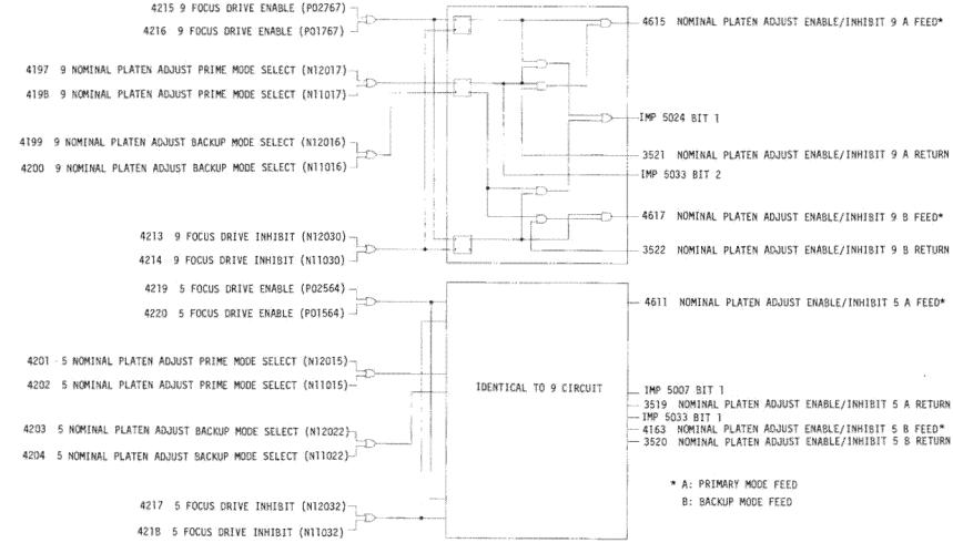
Figure 3.9-32. Nominal Platen Adjust Enable/Inhibit and Mode Select
