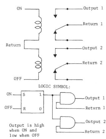
Figure 3.9-17. Latching Relay ON/OFF Control Circuit Logic Representation
