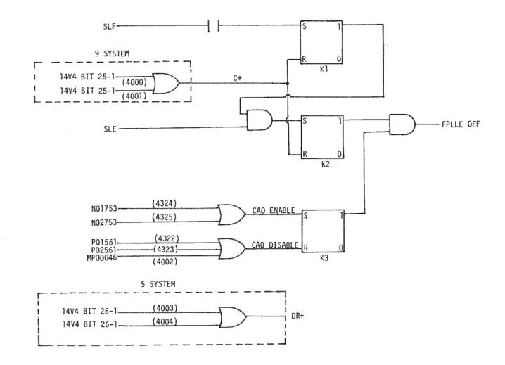
Figure 3.9-50. Camera Automatic Off Logic Diagram
