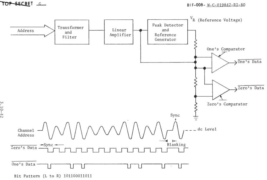
Figure 3.10-25. Address Receiver Block Diagram
