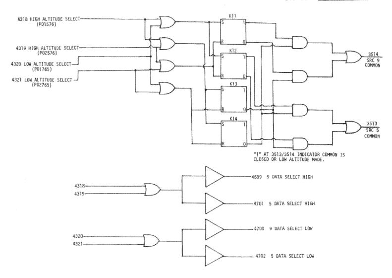
Figure 3.9-49. High/Low Altitude Select SRC Common and Data Lamp Select
