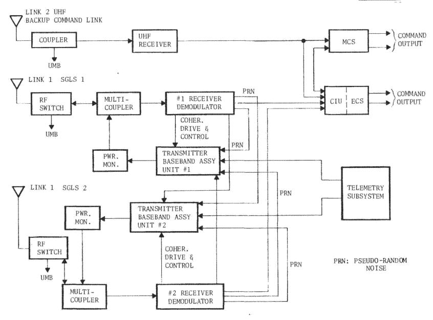
Figure 3.9-2. Vehicle Communications Block Diagram
