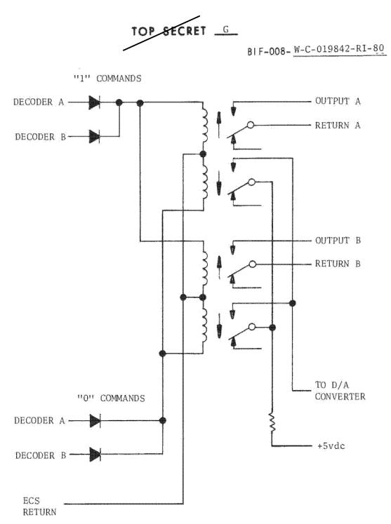
NOTE: Commands may also be coupled through optical isolators, in which case the return line will be the 24.5v power return.
