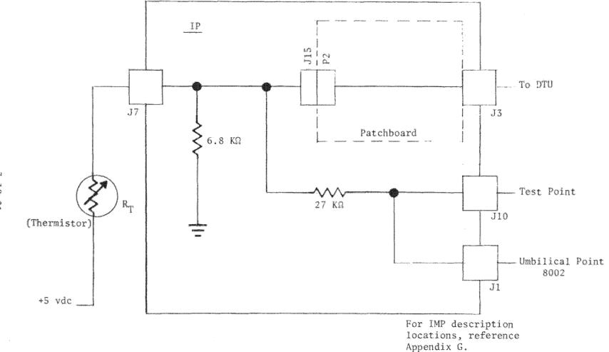
Figure 3.10-10. IMP 5114 Processing Circuit
