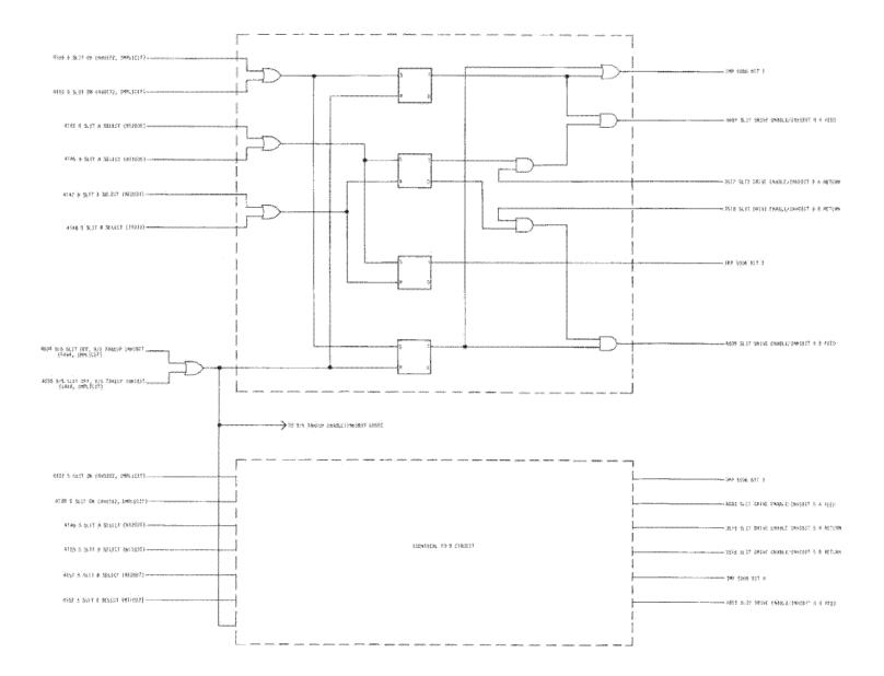
Figure 3.9-35. 9 and 5 Slit Drive Enable/Inhibit/Select
