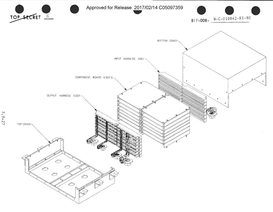
Figure 3.9-13. Command Processor Assembly
