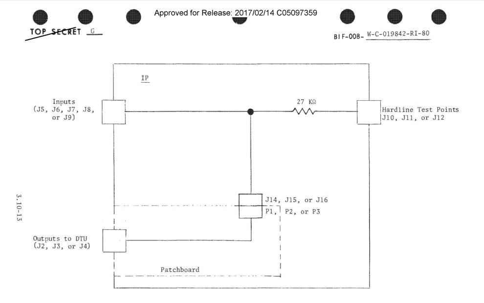
Figure 3.10-5. Typical Preprocessed Analog Signal IP Circuit
