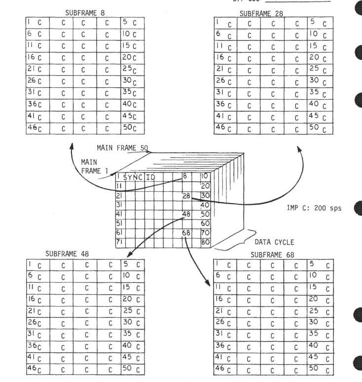
Figure 3.10-46. Format Example: 200 sps Monitor 3.10-92
