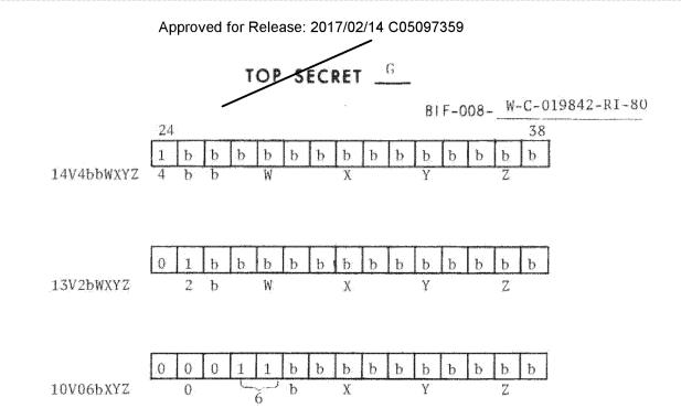
Figure 3.9-7. ECS 14V, 13V, and 10V VSPC Octal Codes Examples of other variable words available to the PPS/DP EAC are 4V0172bZ, 4V0152bZ and M6V002YZ (MCS command). Additional VSPC's in the ECS and MCS are assigned to the satellite control section (SCS).
