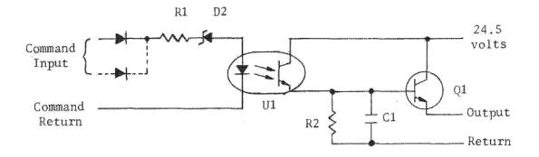
Figure 3.9-18. Basic Optical Isolator and Pulse Circuit
