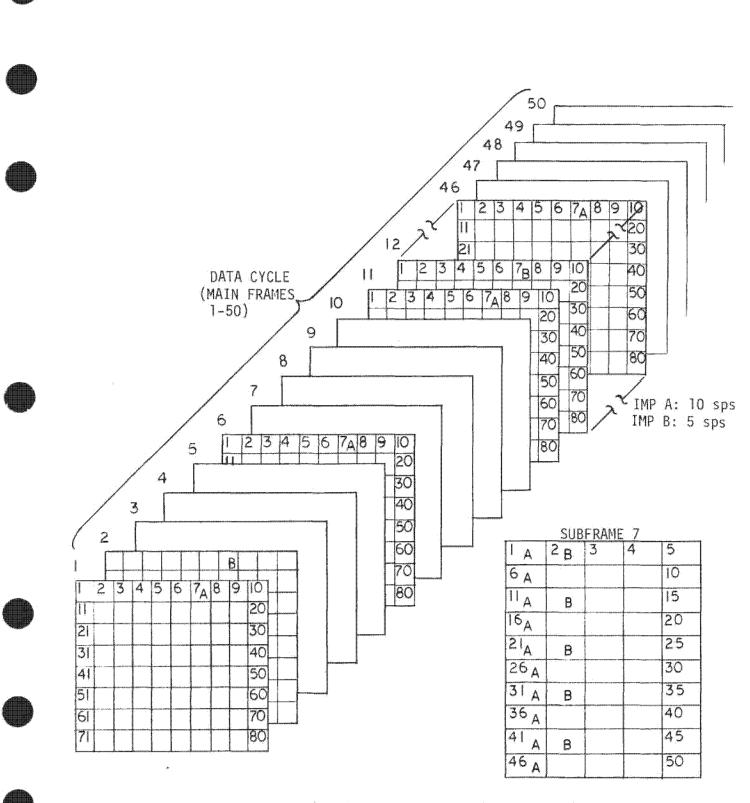
Figure 3.10-45. Format Example: 10 sps and 5 sps Monitors
