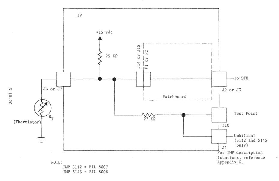
Figure 3.10-9. Typical IP Processing Circuits: IMP's 5111, 5112, and 5145
