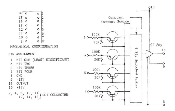
Figure 3.9-19. Instrumentation Digital-to-Analog Converter
