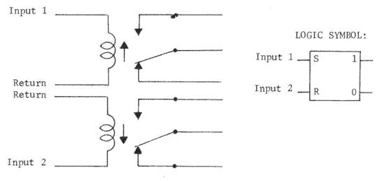
Figure 3.9-16. Latching Relay Logic Representation
