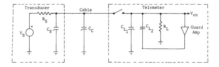
Figure 3.10-53. Sampling Transient Error Source
