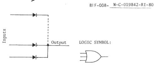
Figure 3.9-15. Command Input Diode OR Gate
