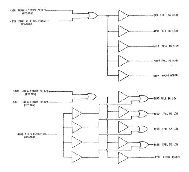
Figure 3.9-48. High/Low Altitude Select FPLL Altitude Range and Focus Normal/Modify
