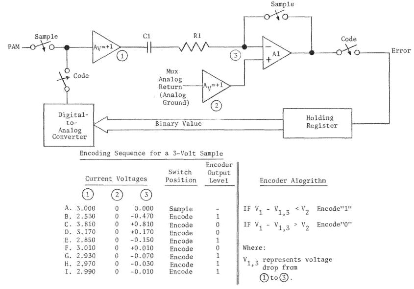
Figure 3.10-29. Analog-to-Digital Converter - Block Diagram, Sample/Encode Algorithm and Encoding Example
