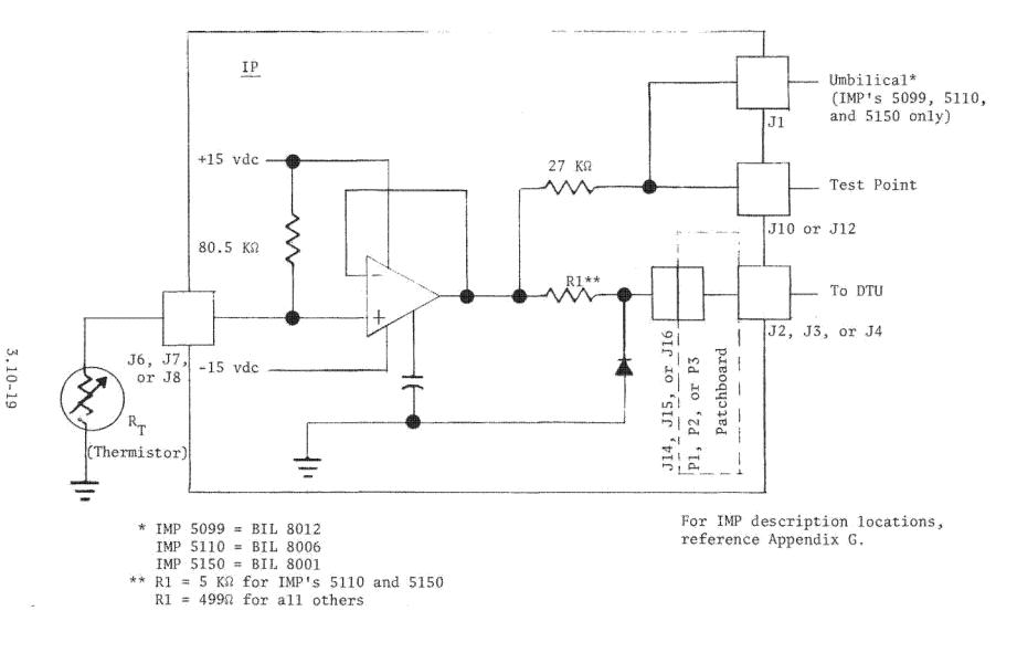
Figure 3.10-8. Typical Processing Circuitry: IMP's 5099, 5110, 5113, 5115, 5120, 5150, 5155
