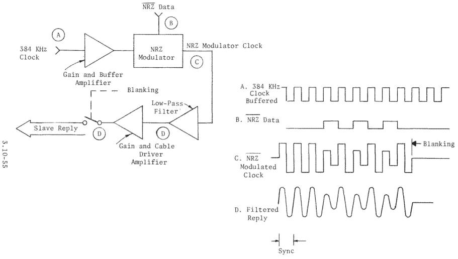
Figure 3.10-31. Reply Modulator
