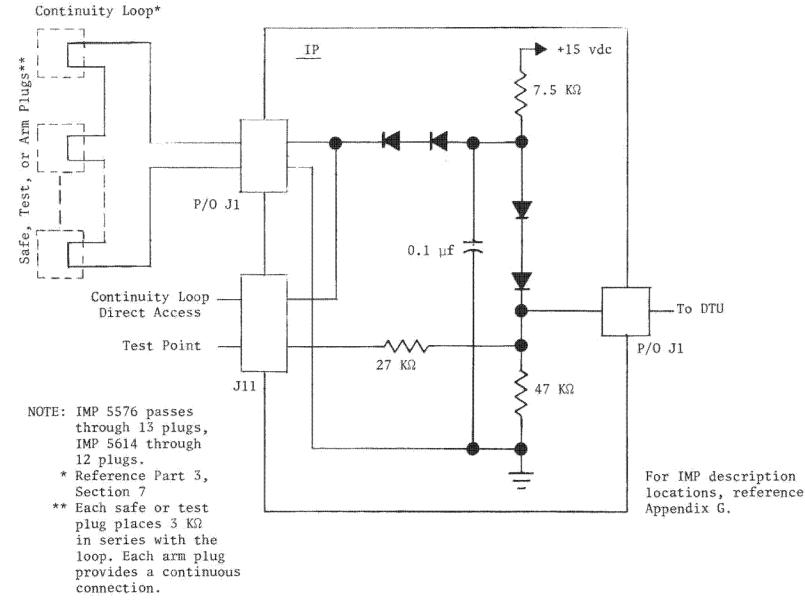
Figure 3.10-15. Typical IP Processing Circuit: IMP's 5576 and 5614
