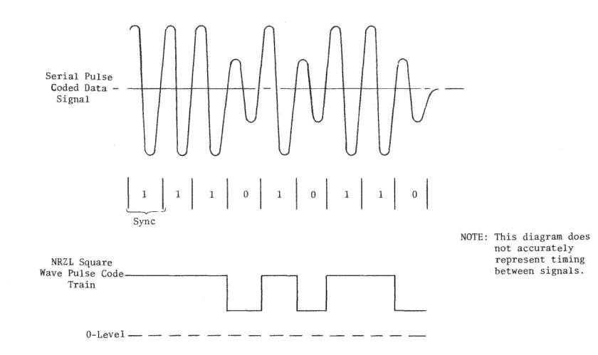
Figure 3.10-43. Binary Coded Square Wave NRZL Pulse Code Train
