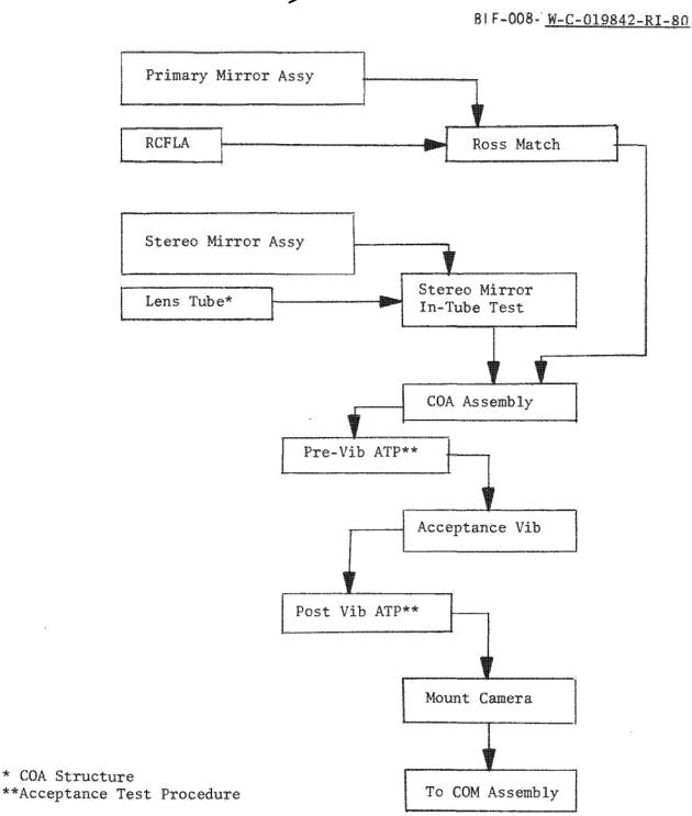
Figure 4.4-5. COA Assembly and Test Flow
