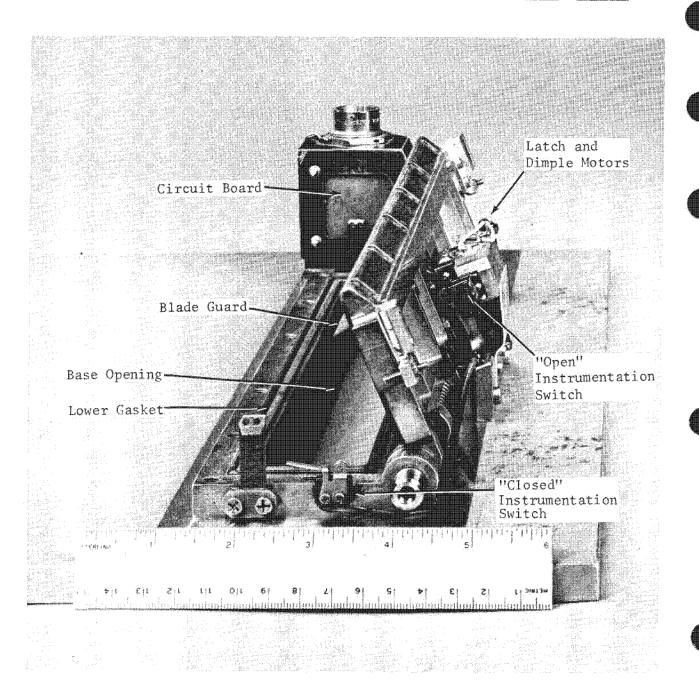
Figure 3.11-3. Cutter/Sealer Assembly (Open)
