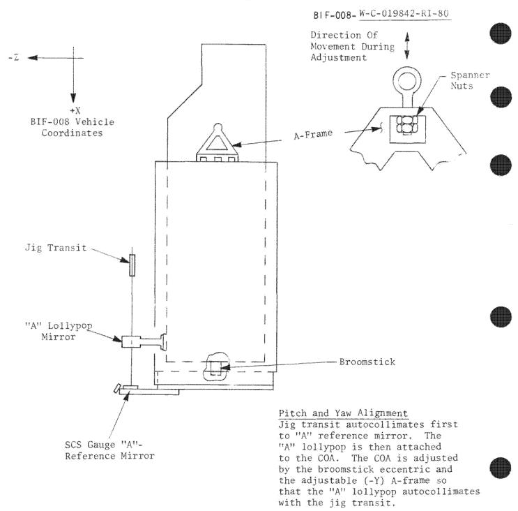
Figure 4.3-11. Optical Axis To Vehicle Axis Pitch And Yaw Alignment
