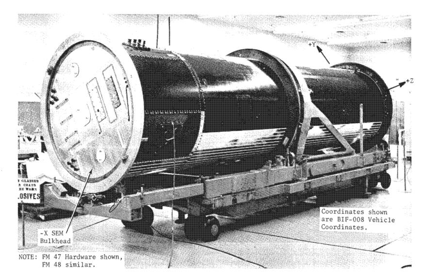
Figure 4.3-16. SEM/COM Assembly
