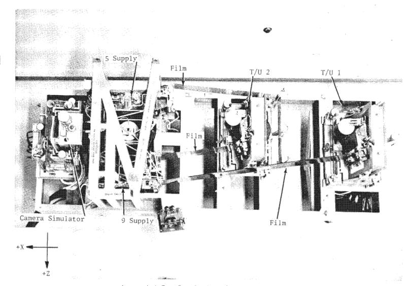
Figure 4.4-7. Supply Assembly Test Set
