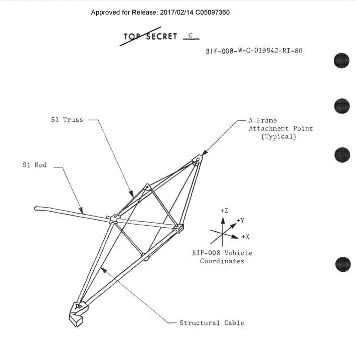
Figure 3.13-2. S1 Rod and Truss Assembly
