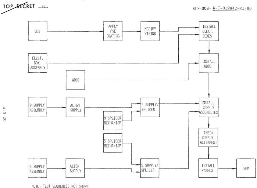
Figure 4.3-12. SEM Assembly Flow
