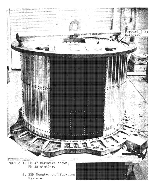
Figure 4.3-13. Supply Electronics Module (-Z View)
