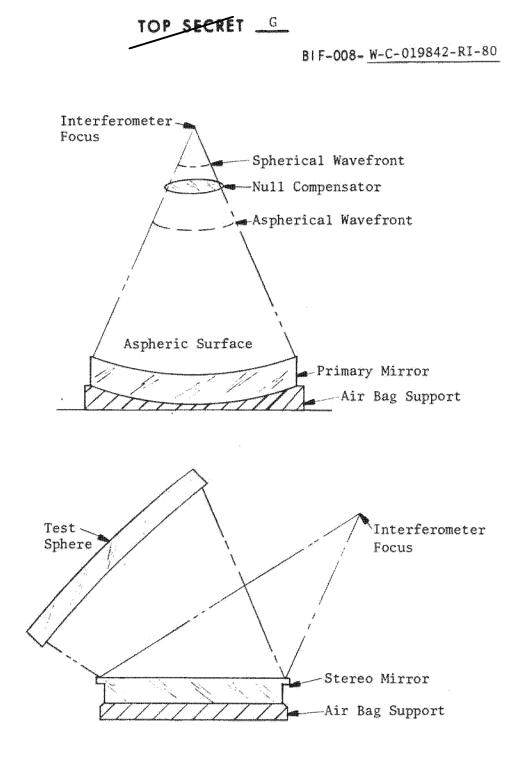
Figure 4.4-1. On-Back Primary and Stereo Mirror Tests
