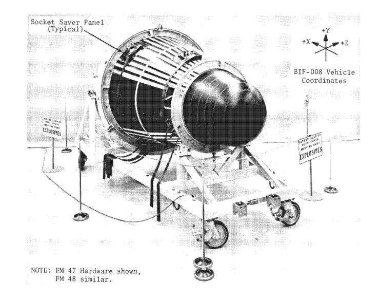
Figure 4.3-15. Dual Recovery Module
