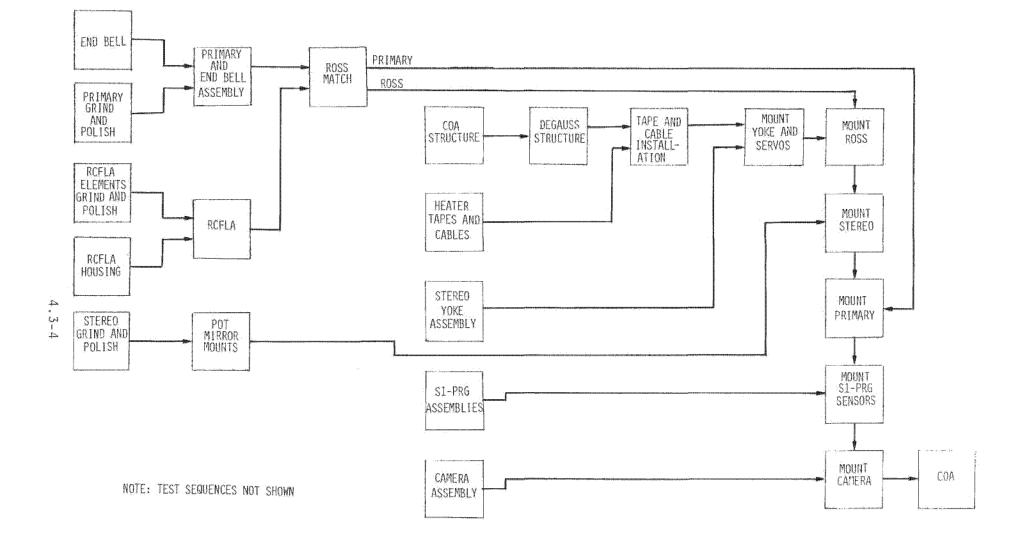
Figure 4.3-2. COA Assembly Flow
