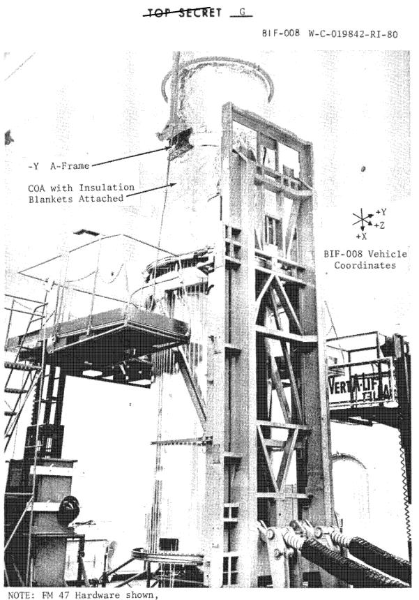
NOTE: FM 47 Hardware shown, FM 48 similar. Figure 4.3-8. Mating COA to Aft Barrel 4.3-14
