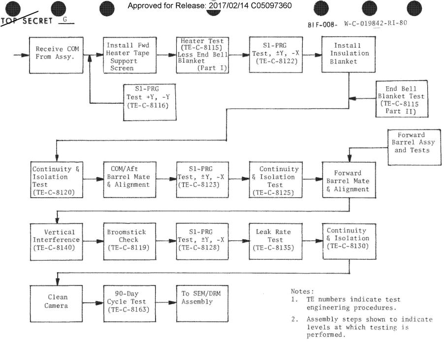
Figure 4.4-8. COM Assembly and Test Flow
