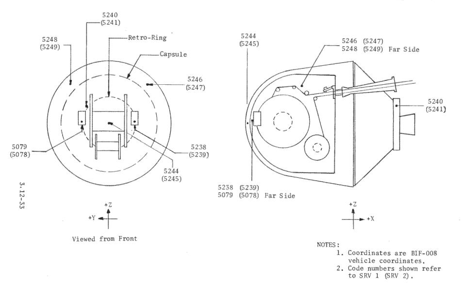
Figure 3.12-10. SRV Temperature Sensor Locations
