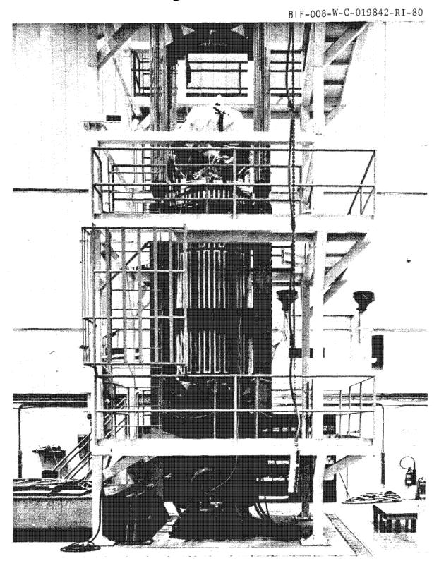
Figure 4.4-4. COA on Vibration Fixture
