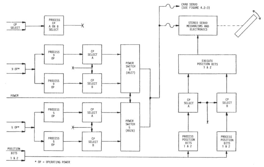
Figure 4.2-2. Stereo Servo Redundancy
