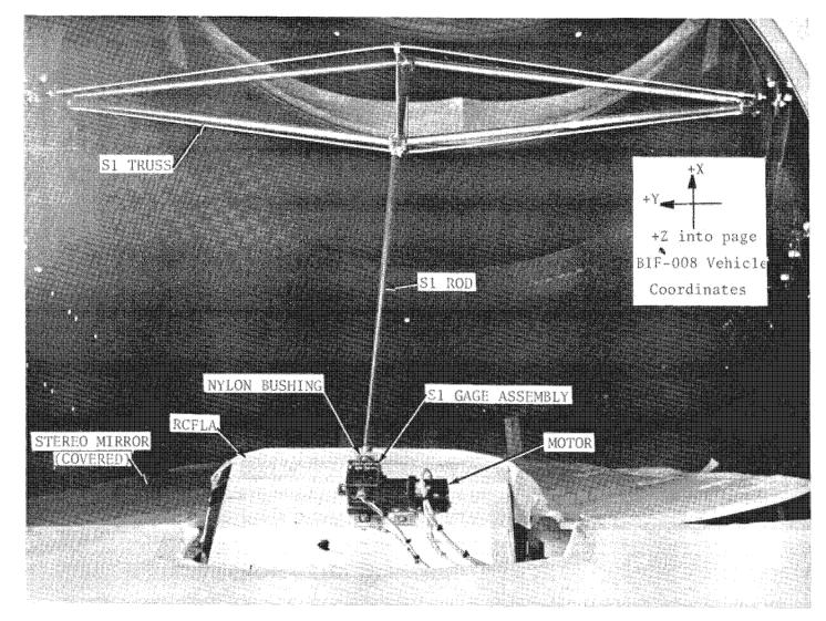
Figure 3.13-1. S1 Sensor Assembly
