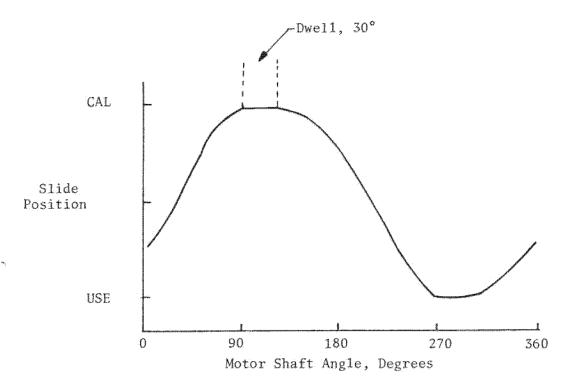
Figure 3.13-7. Slide Input-Output Position Relation
