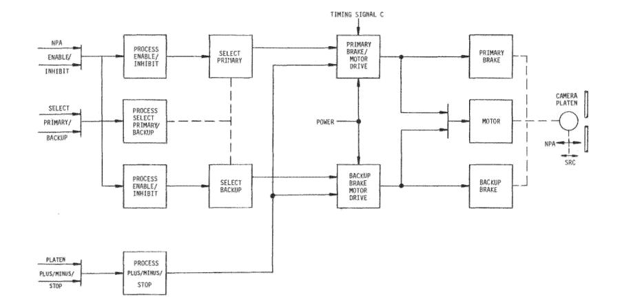
Figure 4.2-8. NPA Subsystem (9 & 5 Identical)
