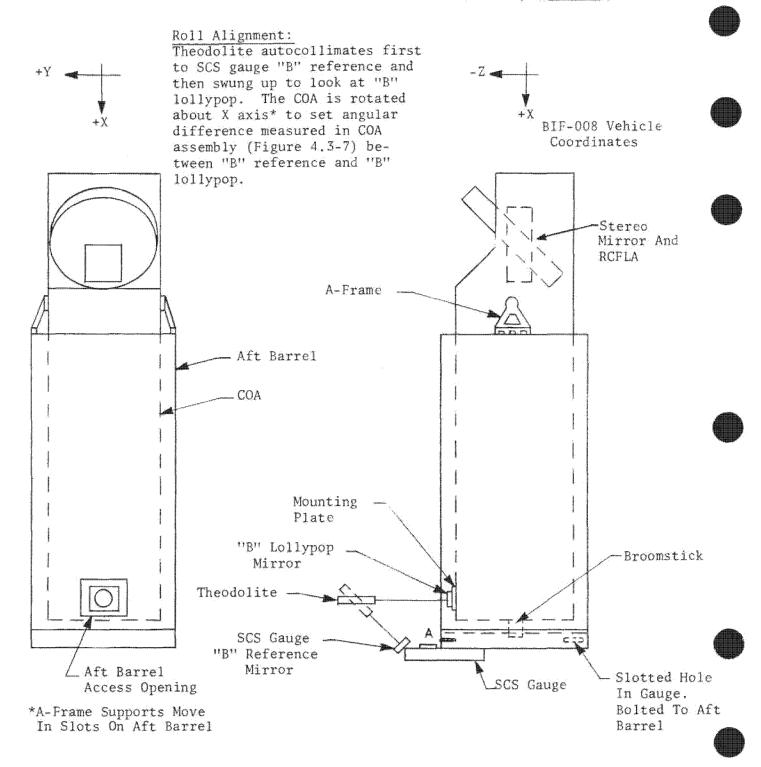
Figure 4.3-10. Optical Axis To Vehicle Axis Roll Alignment
