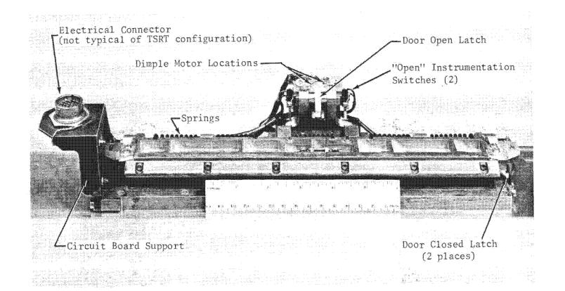
Figure 3.11-2. Cutter/Sealer Assembly (Partially Closed)
