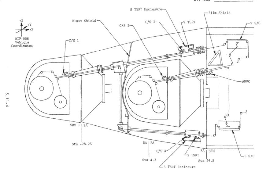
Figure 3.11-1. Cutter/Sealer and Splicer Mechanism Locations
