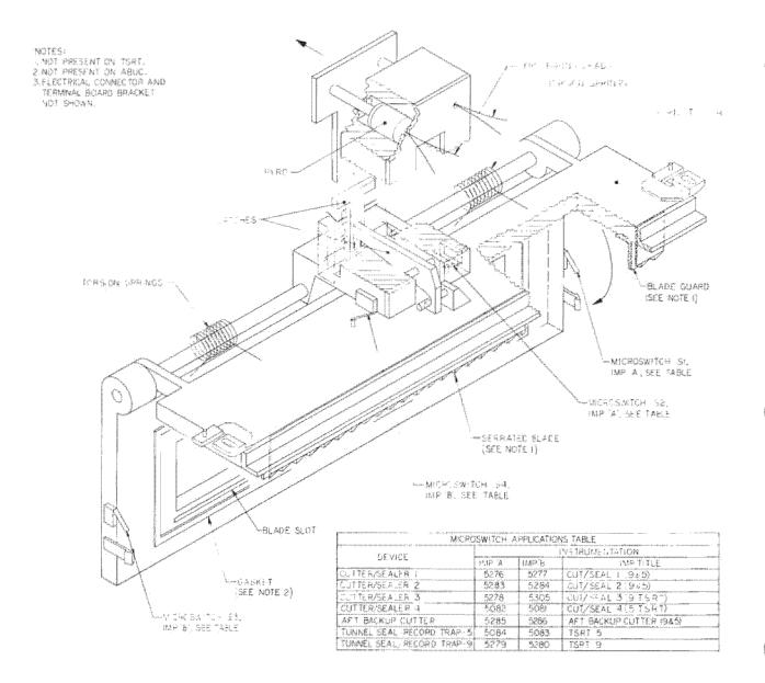
Figure 3.11-5. Typical Cutter/Sealer Device
