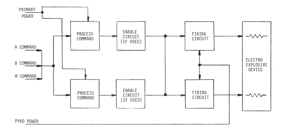
Figure 4.2-1. Initiator Subsystem (Typical)
