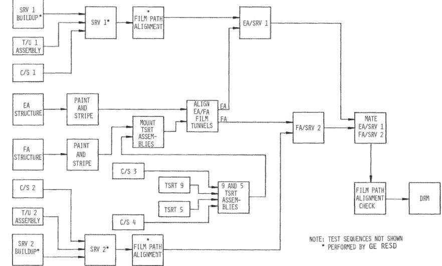
Figure 4.3-14. DRM Assembly Flow
