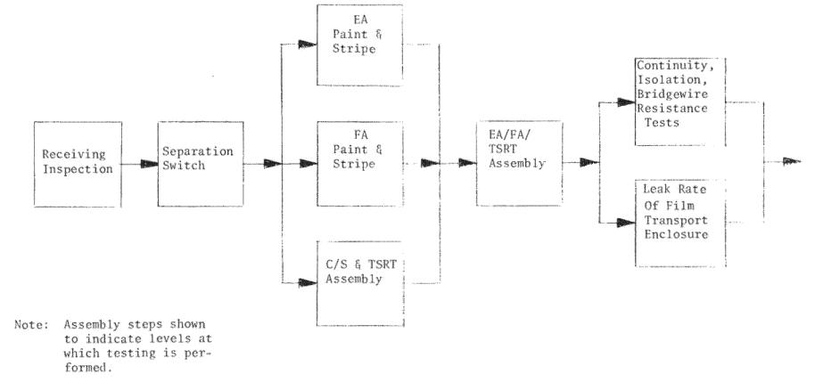
Figure 4.4-10. Assembly Flow and EA/FA/TSRT Test
