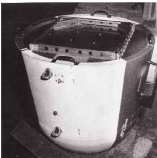
Figure 87. Corona nose cone, August 1959. Note the handle on the right and the drop-aircraft mounting lugs on the left. This nose cone was used to test recovery system effectiveness. Photo courtesy of GE/U.S. Air Force.
