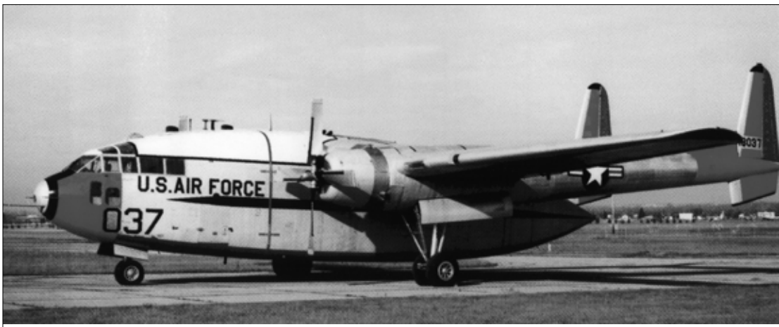
Figure 21. The United States Air Force C-119J #037 responsible for “hooking” the parachute lowering the Discoverer 14 satellite. Photo courtesy of the U.S. Air Force.
