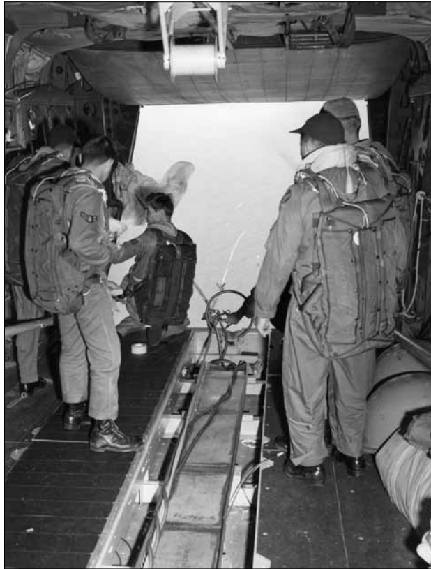
Figure 32. A practice/recovery test where the crewmembers are erecting the recovery poles to reel in the capsule. Photo courtesy of GE/U.S. Air Force.
