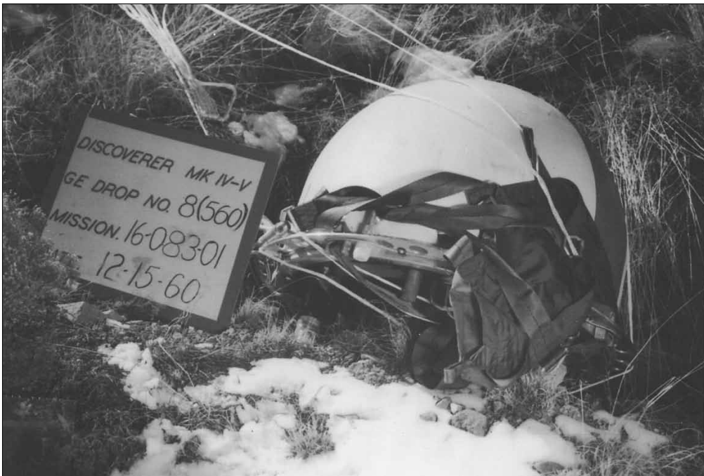
Figure 97. Close-up picture of drop test number 2; note the parachute is not opened. Photo courtesy of GE/U.S. Air Force, 1959.
