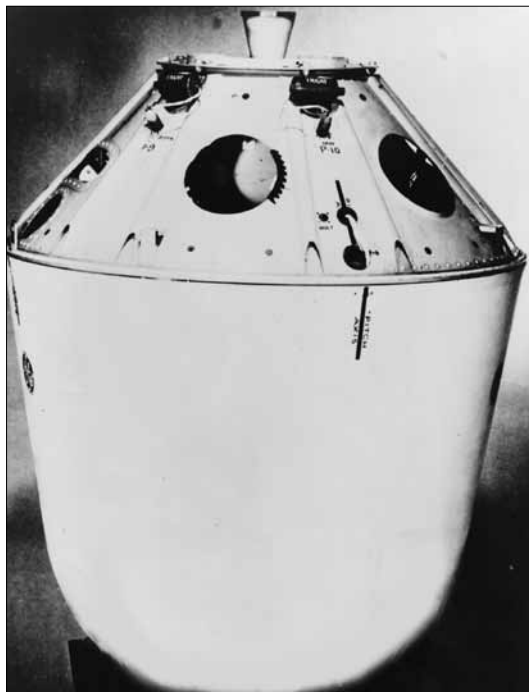
Figure 118. External picture of the SRV. The spherical cone dominating the bottom half is the reentry shell. Photo courtesy of GE/U.S. Air Force.
