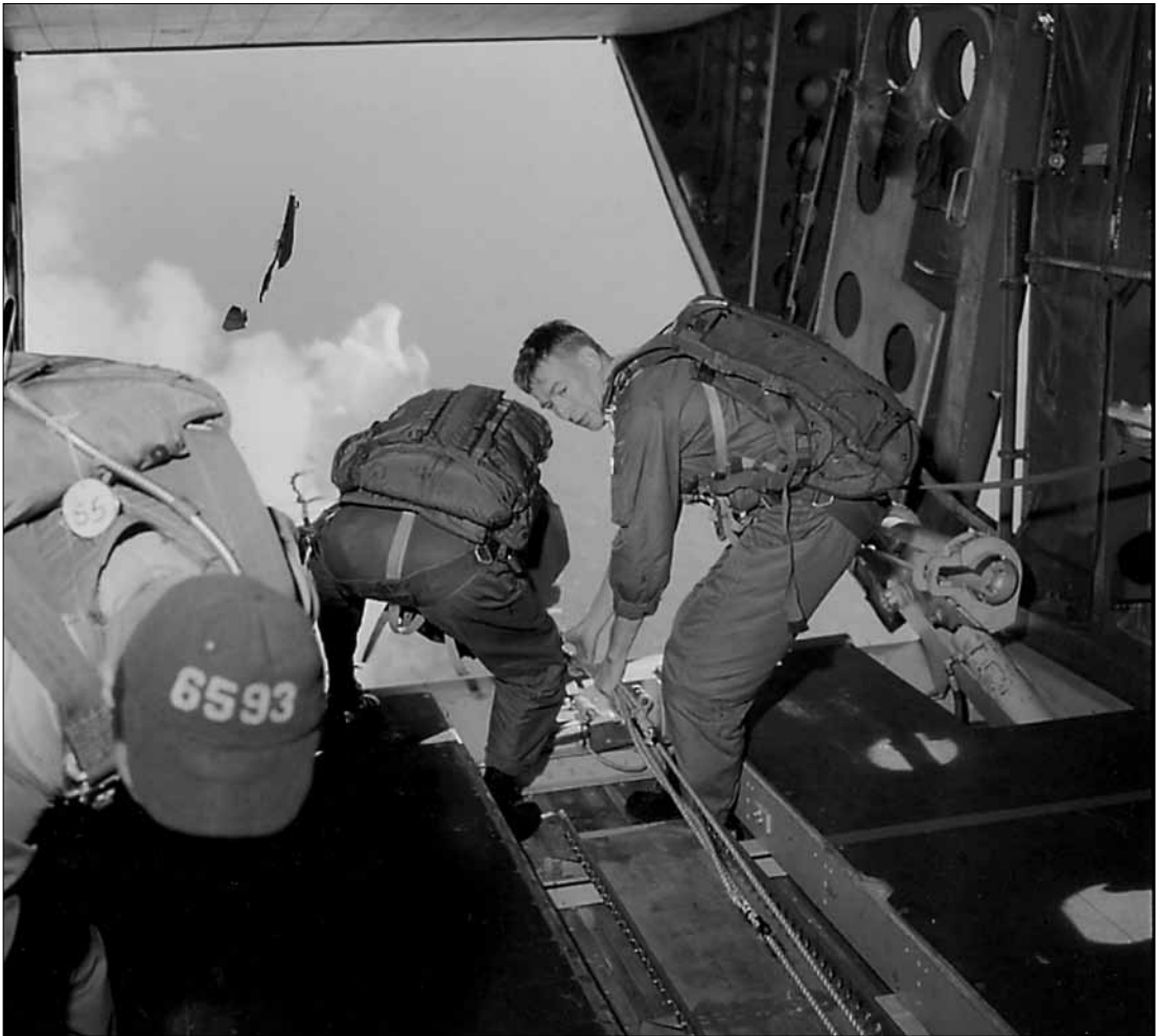
Figure 31. A practice recovery test over the Pacific Ocean near Hickam AFB, Hawaii. The first part of the loop is being reeled on board by the crew. Photo courtesy of GE/U.S. Air Force.
