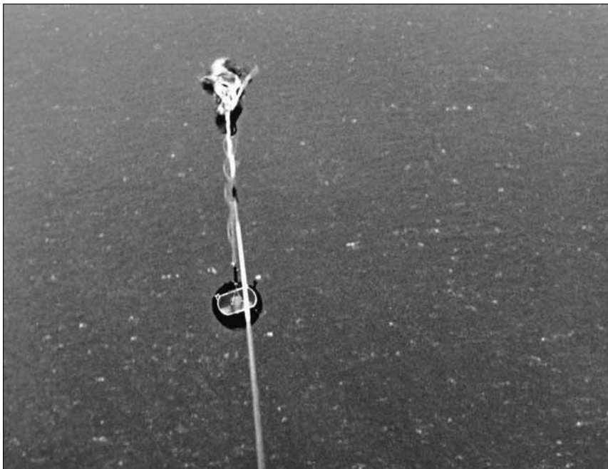
Figure 33. The recovery of Discoverer 14. The capsule and chute are nearing the rear of the aircraft. Note the charcoal black top of the capsule, soot from reentry, and clean center where the parachute cover door has been ejected. Photo courtesy of GE/U.S. Air Force.
